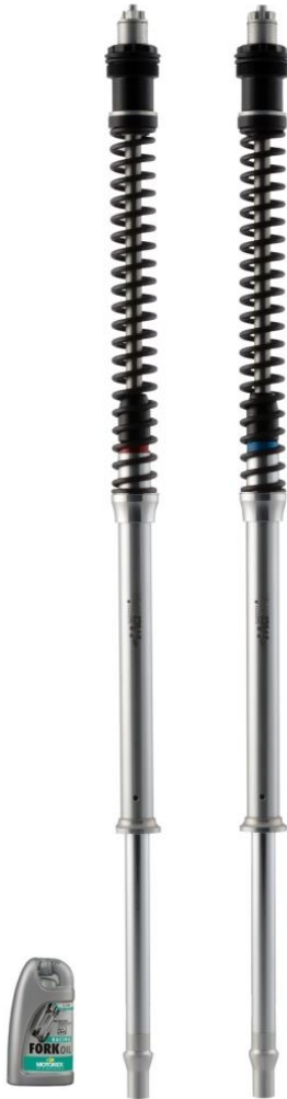
F15K "quad valve system" fork kit
