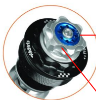
F25SA sealed fork cartridge kit Quad-valve asymmetric system
