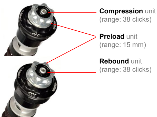
F20K cartridge fork kit Quad-valve asymmetric system
