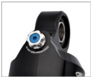
Nitrogen gas valve
