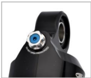
Nitrogen gas valve
