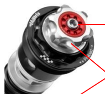
F25R fork kit quad-valve asymmetric system
