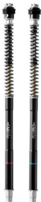
F25SA fork kit sealed asymmetric system
