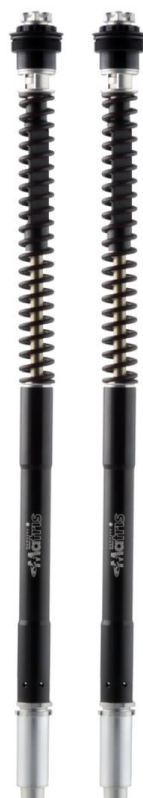
F25R fork kit quad-valve asymmetric system
