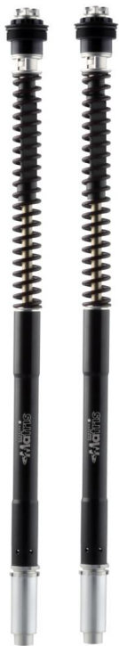
F25R Quad-valve asymmetric system
