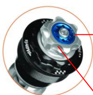
F25SA sealed fork cartridge kit Quad-valve asymmetric system
